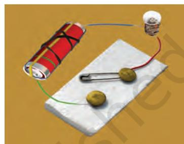
**Fig 12.9** An electric circuit with a switch
