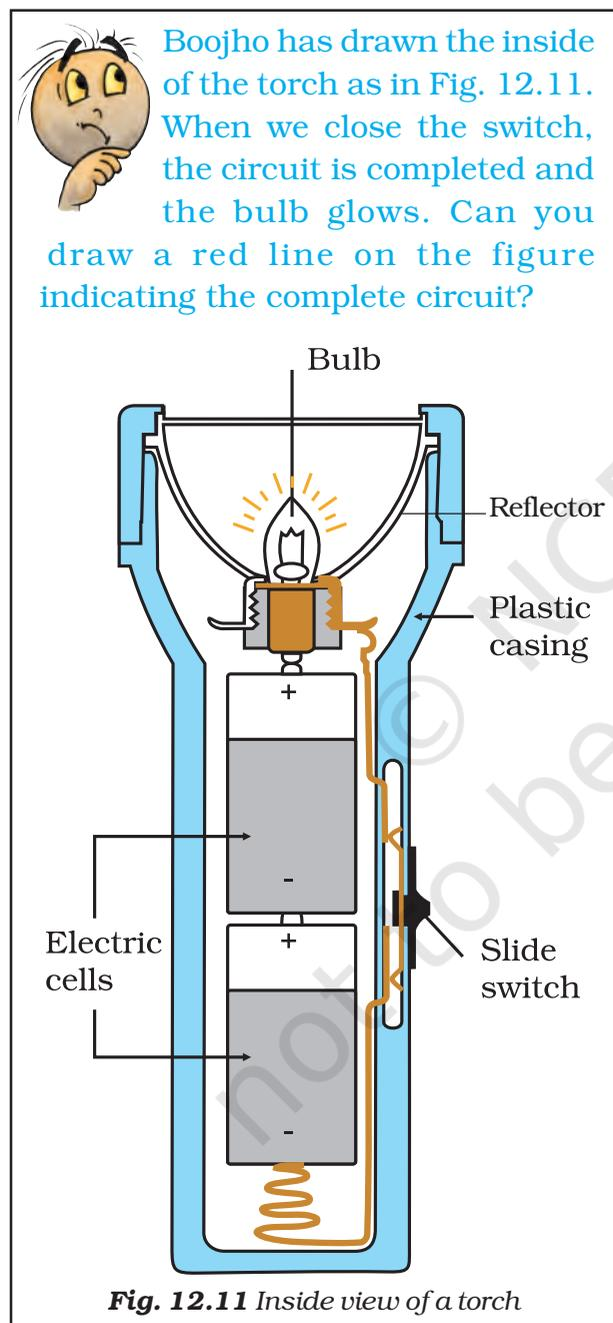
**Fig. 12.11** Inside view of a torch
